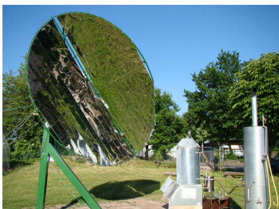
Figure 10 The solar based distillery for essential oils extraction from medicinal plants presented by Waseem Amjad, University of Kassel, Germany, at SuNEC 2013, Santa Flavia, Sicily, September 12, 2013. A video of the system during a real distillation, courtesy of Professor A. Munir, University of Agriculture Faisalabad-Pakistan, can be seen at the URL: http://shorturl.at/iosK6
