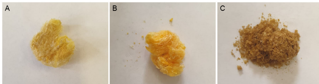
FIGURE 1 | Citrus IntegroPectin samples sourced via AC from industrial CPW following obtained by freeze-drying the precursor solution after 24 h dialysis: (A) lemon IntegroPectin, (B) sweet orange IntegroPectin, (C) red orange IntegroPectin. AC = Acoustic cavitation; CPW = citrus processing waste.
