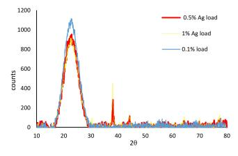
Figure 1. XRD patterns of 70:30 SilverSil with different silver loading (1 %, 0.5% and 0.1%).
