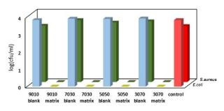
**Figure 4.** Antibacterial activity of different (10%, 30%, 50% and 70% methyl-modified) SilverSil xerogels against *S. aureus* (green bars), and *E. coli* (blue bars). The activity of different blank matrices and of the control solution is also plotted (red bars).
