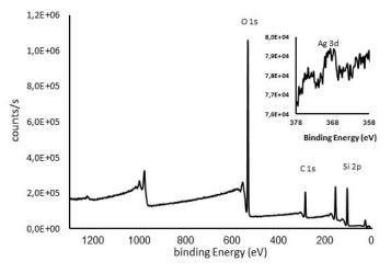
Figure 2. XPS spectrum of 70:30 SilverSil xerogel; inset: Focused scan for Ag peak.
