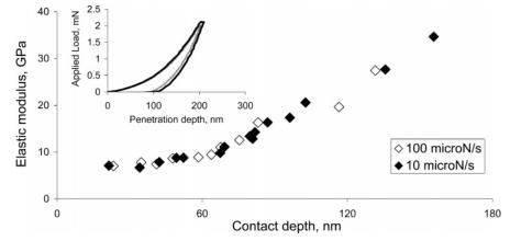
Figure 3. Elastic modulus of the Si100Me film undergoing nanoindenation at different speeds and, in the inset, loading curves for the Si50Me film at different speeds (black line, 7 mN/s; gray line, 70 mN/s).
