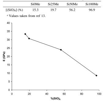
Figure 10. Correlation between the elastic modulus and the percentage of  $(SiO)_6$  rings in the organosilica matrix.
