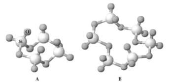
**Figure 9.** Schematic diagram of the more common types of primary cyclic arrangements of the structural units,  $SiO_4$ , in xerogels: (A) four-membered siloxane ring (SiO)<sub>4</sub> and (B) six-membered siloxane ring (SiO)<sub>6</sub>.
