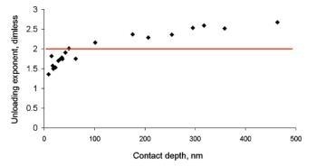
**Figure 7.** Variation of the unloading exponent (*b*) versus contact depth.
