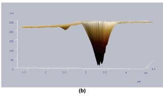
**Figure 6.** At 2 mN nanoindentation of the film surface (here shown for the SiMe25 sample) with deep tip penetration masks the measurements due to the effect of the substrate. (a) and (b) show two different views.
