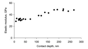
**Figure 5.** Variation of the elastic modulus versus contact depth for the Si5Me film.
