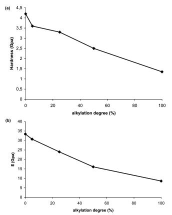
**Figure 8.** Hardness (a) and elastic modulus (b) as a function of the degree of alkylation of the silica matrix in ORMOSIL thin films.
