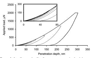
**Figure 4.** Loading–unloading force curves at varying loads between 30 and 2000  $\mu$ N for the Si50Me film.
