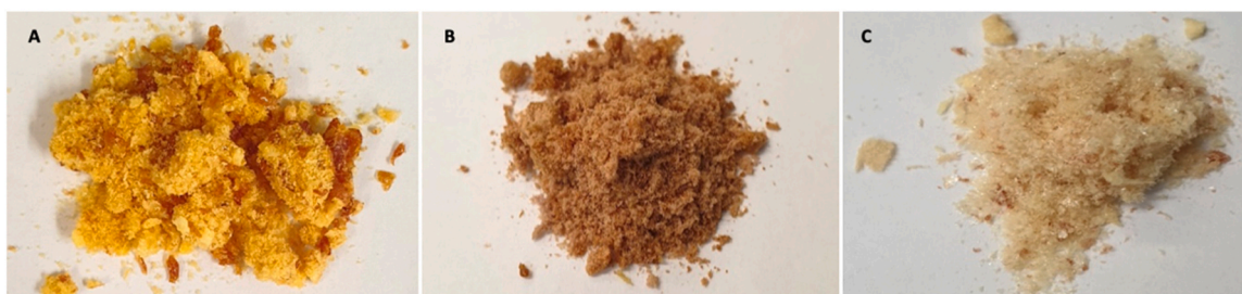
Fig. 1. Sweet orange (A), red orange (B), and lemon (C) IntegroPectin sourced from industrial citrus processing waste by acoustic cavitation.
