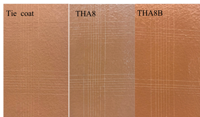
Fig. 7. Adhesion-cross cut test of commercial tie coat, THA8 and THA8B topcoats.
