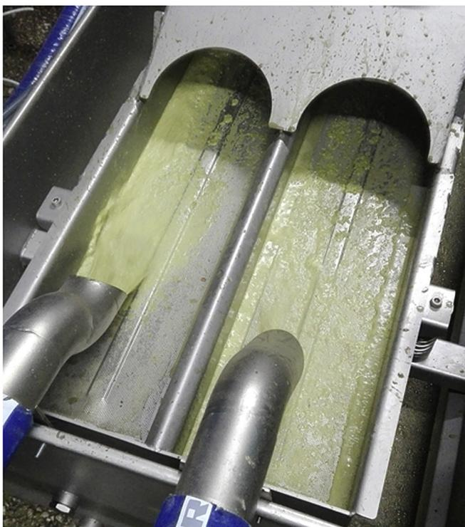
Fig. 1. Water phase output of the three-phase vertical centrifugation.
