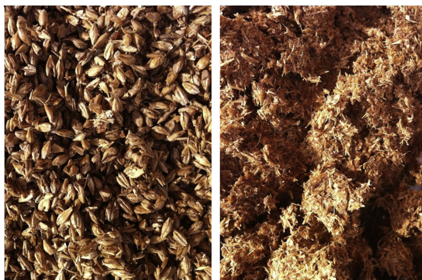
Fig. 2. Malt particles after a traditional brewing process (left) and after hydrodynamic cavitation processing (right).
