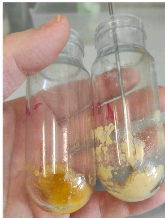
Fig. 5. Bitter orange IntegroPectin (left) and red orange IntegroPectin (right) after flavonoid extraction with aqueous EtOH at room temperature. [Copyright: The Authors, 2022. Reproduced from Scurria et al., 2022, Creative Commons CC BY 4.0 Attribution License].
