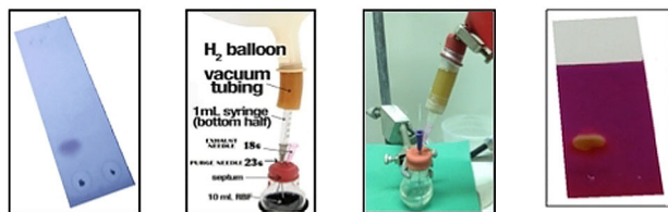
Figure 2. Progress of methyl trans -cinnamate hydrogenation mediated by SiliaCat Pd(0) followed by thin layer chromatography. [Image courtesy of Prof. Kenneth O'Connor, Marshall University].
