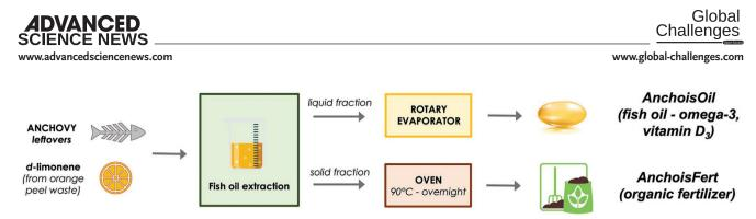
Scheme 1. Overall upgrading process of anchovy fillet leftovers converted into AnchoisOil and AnchoisFert.
