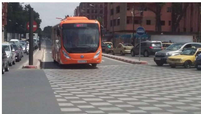
Figure 2. The roads of Marrakech, Morocco, have hosted 15 electric buses since 2017. Each bus runs with overhead cables outside the city center but each bus runs only on battery energy within the city. Photo reproduced with permission from https://www.skyscrapercity.com/show-thread.php?t=1468062&page=20 .
