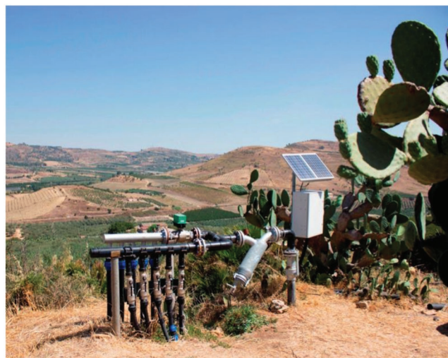
Figure 5. One of the 13 solar-powered sensor and actuator systems controlling solar-powered irrigation in a 100 ha Opuntia ficus-indica plantation in Sicily, Italy. (Image courtesy of Agrowireless).
