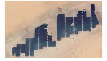
**FIGURE 1** The Noor Abu Dhabi 1.177 GW solar park in Sweihan, UAE, comprises 3.2 million PV modules. [Photograph via Google Earth, June 2019]
