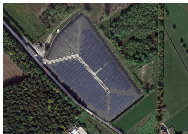
Figure 3. Tiretta landfill near Treviso, Italy. The CIGS solar modules on top of the geomembrane are clearly visible. Satellite photograph using Google Earth, 2017.
