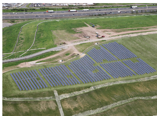
Figure 6. Hartford landfill in Connecticut hosting a 1 MW photovoltaic plant with rigid modules on top of synthetic turf. Image of Connecticut Materials Innovation and Recycling Authority, reproduced from Ref. [21], with kind permission.
