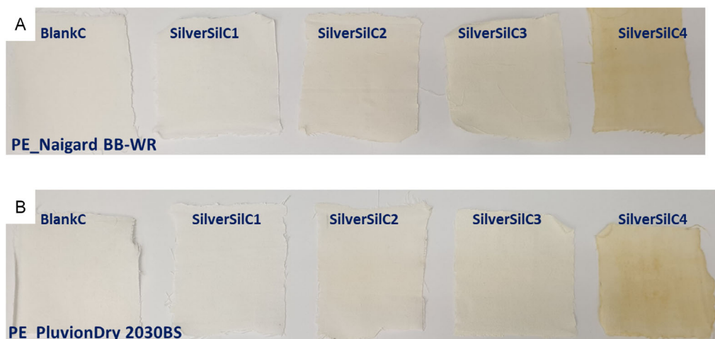
Figure 3. Polyester fabrics after coating with 3.5% of BlankC and SilverSil xerogels (doped with different amounts of Ag NPs) dispersed in A) Naigard BB-WR and B) Pluvion Dry 2030 BS.
