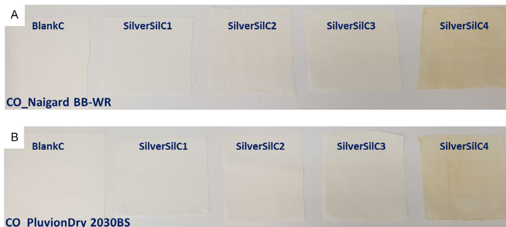
Figure 2. Cotton fabrics after coating with 3.5% of BlankC and SilverSil xerogels (doped with different amounts of Ag NPs) dispersed in A) Naigard BB-WR and B) Pluvion Dry 2030 BS.
