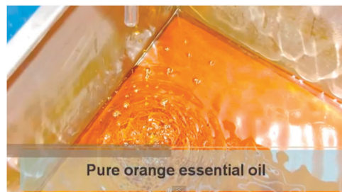
Fig. 3 Orange essential oil from orange peel obtained at room temperature after centrifugation of the water oil emulsion. [Image courtesy of Fratelli Indelicato Srl.]
