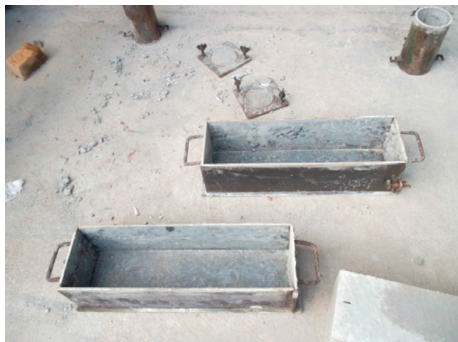
Figure 5. Molds and cylinders with cement residues following stripping of the set cement after 48 h. The mold in front, containing cement added with crude glycerol, is clean. (Photograph by Prof. S. Vásquez.)
