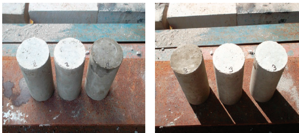
Figure 4. Cylinders of concrete midday (left) and at the end of the same day (right). The slightly coloured cylinders are the samples added with crude glycerol. (Photograph by Prof. S. Vásquez.)
