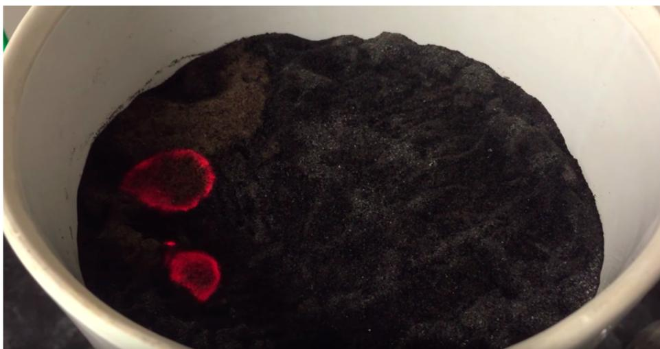
**Figure 1.** SiliaCat Pd<sup>0</sup> kept in a Büchner funnel by filter paper during vacuum drying of added MeOH using a water aspirator under optimized conditions.
