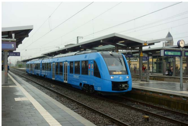
Figure 2. Coradia iLint hydrogen-powered train arriving at Frankfurt-Höchst station on 13 April 2018. (Image courtesy of Matthias Oestreich.)
