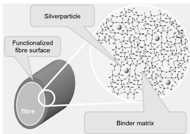
**Figure 1.** Fibre functionalized with a silver-based antibacterial finish incorporating a binder to enhance binding and make the fibres washable. [Reproduced from Ref.14, with kind permission of CHT R. Beitlich].
