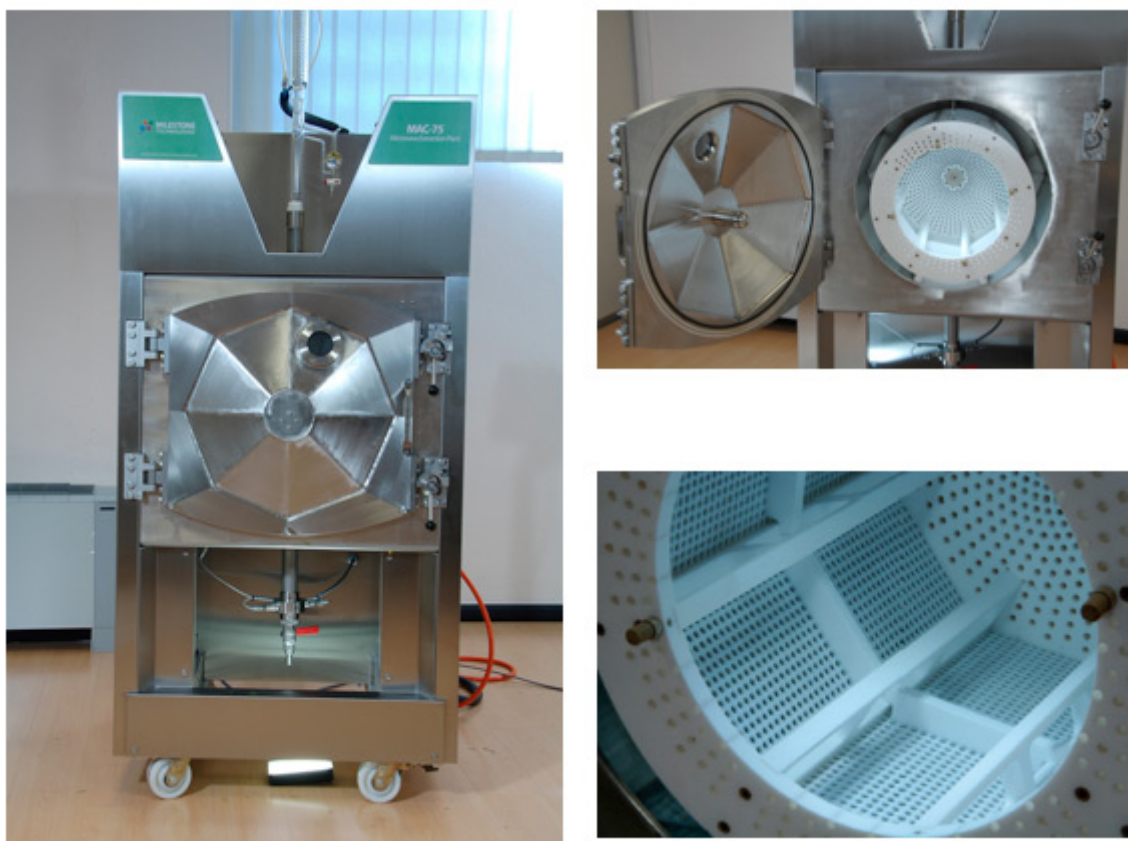
Figure 2. The MAC-75 pilot scale extractor contains four magnetrons ( 4 \times 1500 W, 2450 MHz). The 150 L stainless steel microwave cavity contains a removable PTFE drum that allows up to 75 L of plant material to be loaded. The system automatically adjusts the power delivered if MW absorption, controlled by sensors, is too low. [Photograph of Milestone srl].
