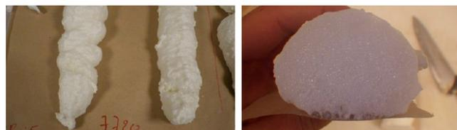
Figure 2. Reference OCF foam 7720 with no added spheres.
