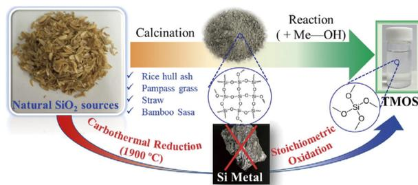
**Scheme 1** One-step direct synthesis of TMOS by reaction of silica and methanol, using a base catalyst and acetal as a dehydrant under carbon dioxide. [Reproduced from Ref. [23], with kind permission]
