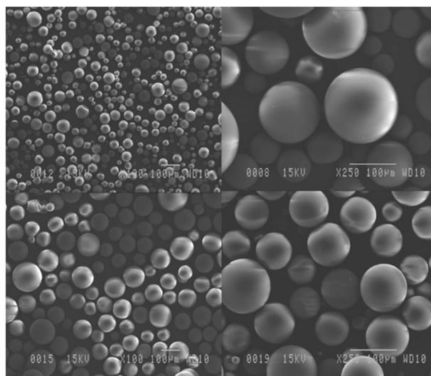
**Fig. 1** SEM images at 100 and 250× magnification of SiliaCat Pd(0),  $d_{50} = 100 \mu\text{m}$ . Lab-scale synthesis (top) and 1.6 kg scaled-up synthesis (bottom). [Reproduced from Ref. 38, Creative Commons CC BY-NC-ND 4.0 license]
