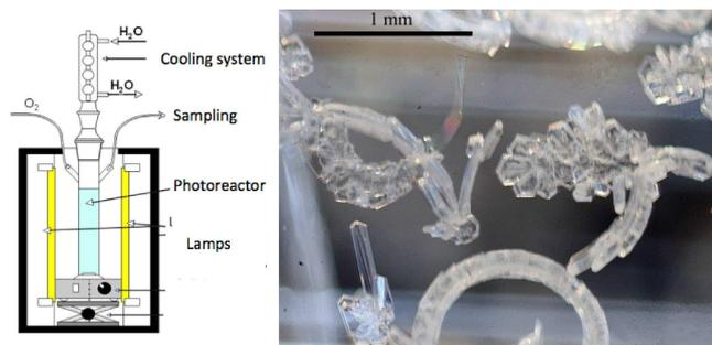
**Figure 1.** Synthesis of vanillin in water by  $\text{TiO}_2$  photocatalytic conversion of ferulic acid under UV irradiation in batch photoreactor (left); vanillin crystals formed by deposition of the permeate vapors (right).
