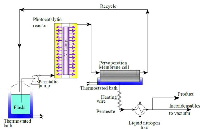
**Scheme 1.** Semi-continuous reaction system integrating photocatalytic reaction and pervaporation unit used to synthesize highly pure vanillin without purification steps. [Reproduced from Ref. [25], with kind permission].
