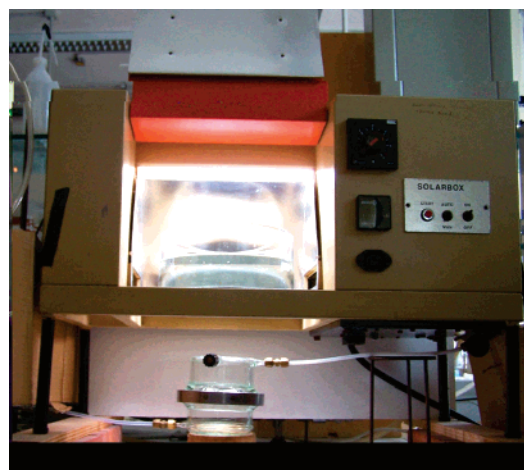
Figure 6. The “Solarbox” reactor employed for carrying out photocatalytic degradation of 2-propanol mediated by doped ORMOSIL/TiO 2 films.
