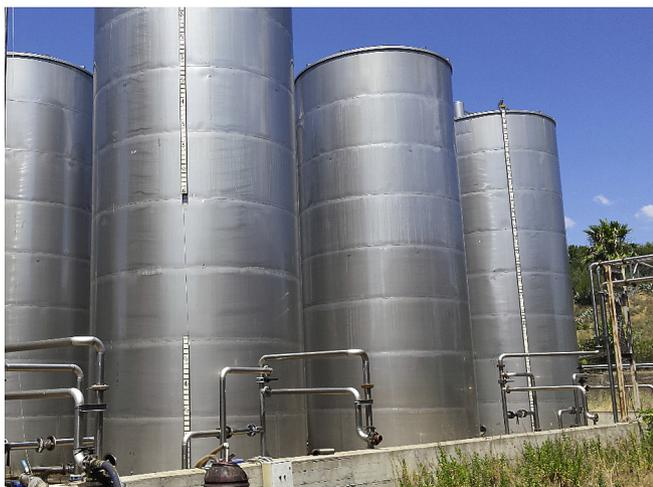
Fig. 3. Silos stocking the olive juice obtained in Sicily in 2016 from a two-phase olive mill.
