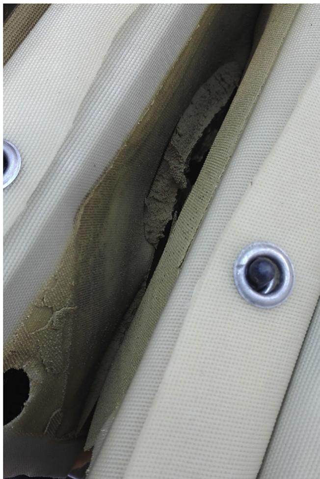
Fig. 2. Solid-cake resulting from the three-phase vertical centrifugation removed using a press filter.
