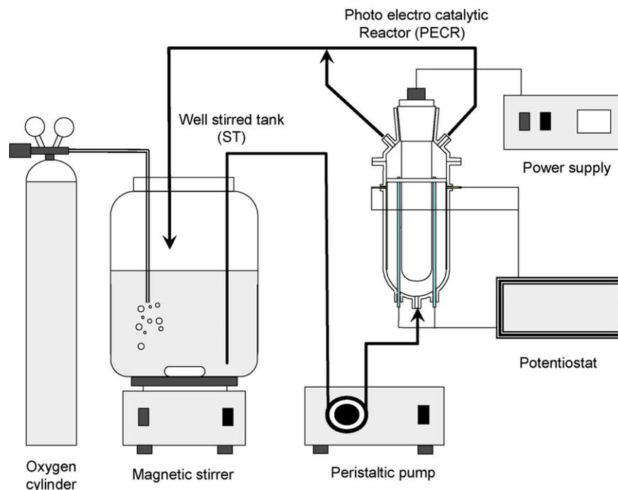
Fig. 1. Set up of experimental apparatus.
