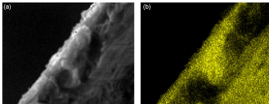
Fig. 6. Cross sectional SEM image (a) and the corresponding EDAX mapping (b) of functionalised anode. Ti is yellow-coloured.
