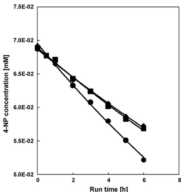
Fig. 7. 4-NP concentration values versus the run time for (◆) photocatalytic, (■) electrocatalytic and (●) photoelectrocatalytic representative runs.
