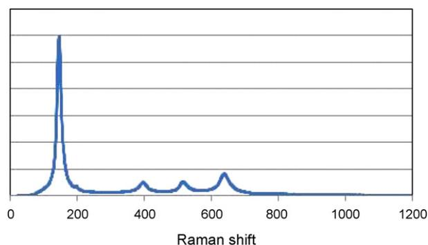
Fig. 4. Raman spectrum of a  $\text{TiO}_2$ -covered graphite rod.
