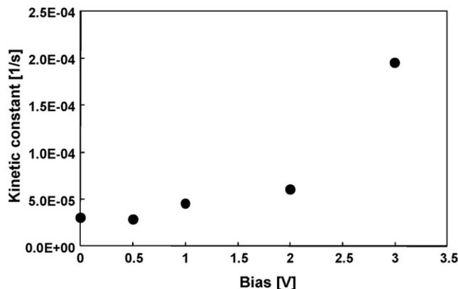
Fig. 10. Kinetic constant,  $k_T$ , vs. applied bias for photoelectrocatalytic oxidation. 4-NP initial concentration,  $7.2 \times 10^{-2} \text{ mM}$ ; flow rate, 3 mL/s.
