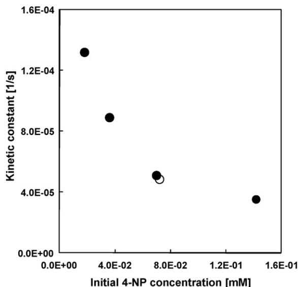
Fig. 11. Kinetic constant,  $k_T$ , vs. initial 4-NP concentration. The empty symbol refers to a run carried out by using air instead of pure oxygen.
