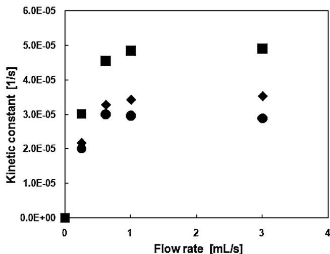
Fig. 8. Kinetic constant,  $k_{\text{T}}$ , vs. liquid flow rate for 4-NP photocatalytic oxidation (●), electrocatalytic oxidation with applied bias of 1 V (◆) and photoelectrocatalytic oxidation with applied bias of 1 V (■).
