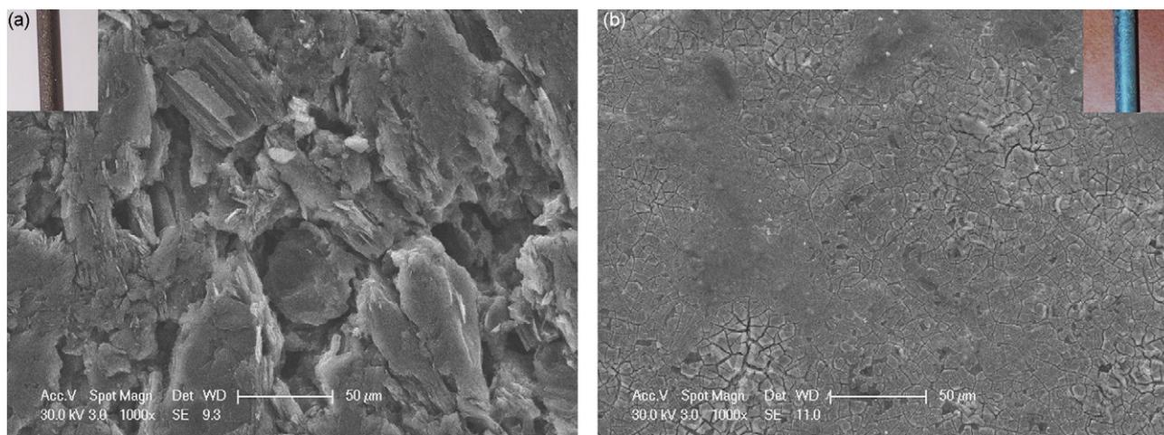
Fig. 5. SEM images and digital photos (insets) of anode's bare (a) and functionalised (b) surface.
