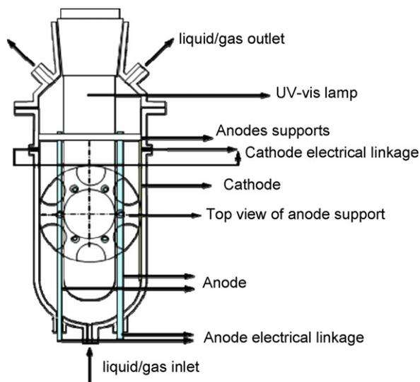
Fig. 2. Scheme of the photoelectrocatalytic reactor (PECR).
