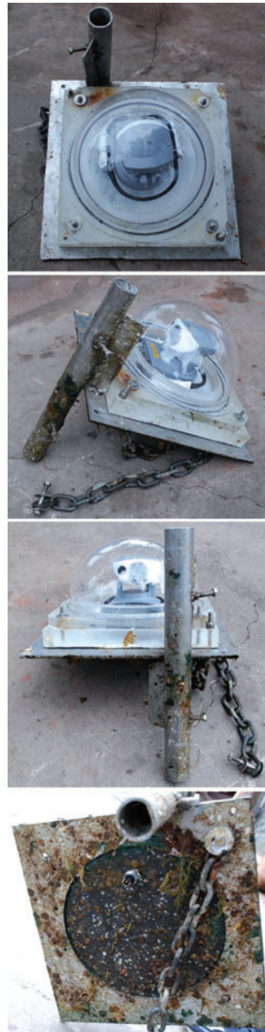
Figure 3. The camera dome and support system after 8 months of continuous deployment underwater at Cala Gadir. Only the upper half of the tube and the top of the plate were treated with AquaFast. The bottom of the plate was not coated. The performance is self-evident.
