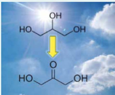
**Scheme 1.** At least two new solar-driven photocatalytic processes have been developed for converting glycerol dissolved in water directly to DHA with oxygen only at room temperature and pressure. [Reproduced from Ref.6, with kind permission].
