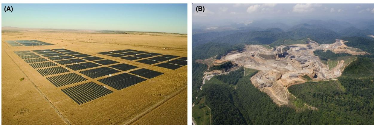
**Figure 4.** Difference in land impact between (A) a solar photovoltaic plant (in Springerville, Arizona: land requirement for PV: 310 m<sup>2</sup>/GWh) and (B) a mountaintop removal coal mining site (in Rawl West, Virginia: Land requirement for surface coal mining: 320 m<sup>2</sup>/GWh) [Reproduced from Ref 18, with kind permission].
