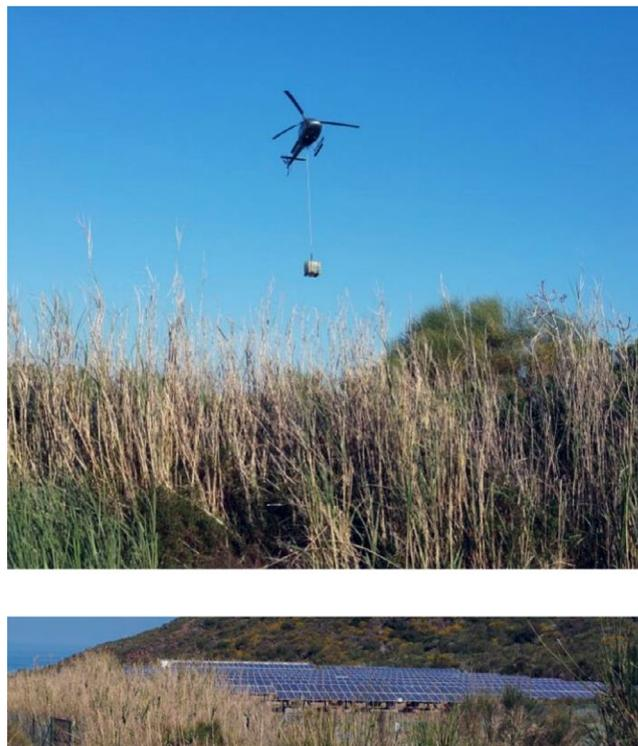
**FIGURE 3** An helicopter (*top*) has been regularly used to bring diesel fuel to the diesel-fueled power generator of the Ginostra village, after the lead-ion batteries coupled to the original 100 kW PV station built in 2004 (*bottom*) quickly went out of use. [Images adapted from: www.remote-euproject.eu, with kind permission]
