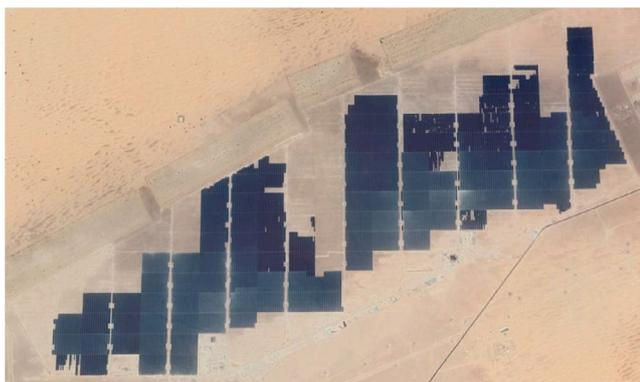
**FIGURE 1** The Noor Abu Dhabi 1.177 GW solar park in Sweihan, UAE, comprises 3.2 million PV modules. [Photograph via Google Earth, June 2019]
