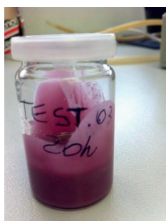
Figure 5. A typical ORMOSIL Alcolgel doped with Au NPs (AuRC1) obtained by the present sol–gel polycondensation process.
