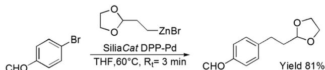
Scheme 5 Heterogeneously catalyzed synthesis of a difunctionalized compound under flow over SiliaCat DPP-Pd [adapted from ref. 27, with kind permission].
