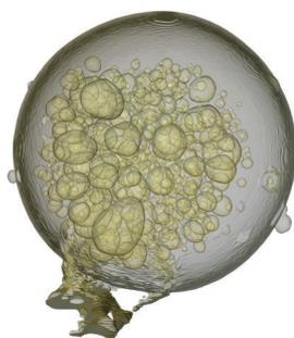
**Fig. 7** X-ray micro-tomography image of a *Ceramisphere* (a trade mark of Ceramisphere Pty Ltd) containing encapsulated limonene clearly seen as liquid bubbles. [Photo courtesy of Dr Sherry Mayo, CSIRO, reproduced with kind permission from ceramisphere.com.]
