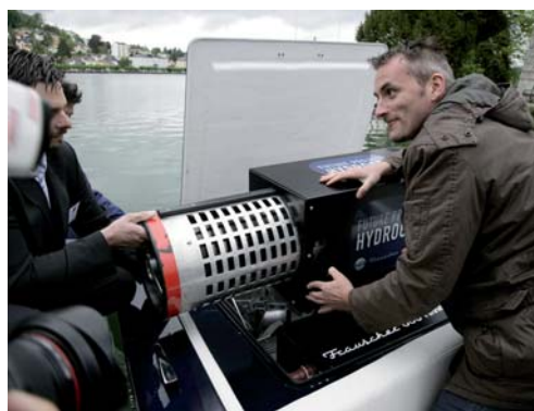
Fig. 7 Re-fuelling of the 600 Riviera Frauscher boat is done in 5 min using a standard 350 bar filler coupling on the one hand plus a simple exchange of an empty cartridge for a full one on the other. (Reproduced from Frauscherboats.com, with permission).
