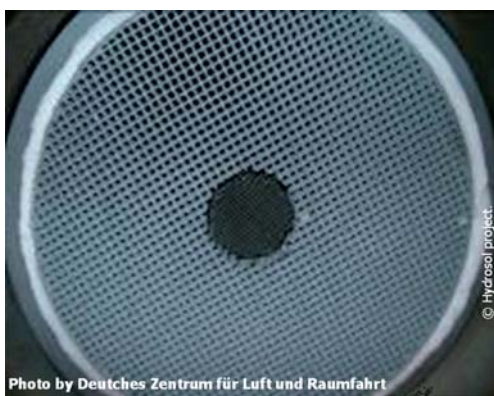
Fig. 13 The monolith channels are coated with active water-splitting materials capable of splitting water vapor passing through the reactor by 'trapping' its oxygen and leaving hydrogen in the effluent gas stream as product pure. (Reproduced from hydrosol-project.org, with permission).
