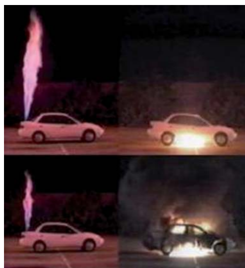
Fig. 4 On the left is a vehicle with a hydrogen tank, and on the right a vehicle with a standard gasoline tank. Both tanks have been deliberately punctured and ignited. The top panel shows the two vehicles 3 s after ignition. The bottom panel shows the two vehicles 60 s after ignition. The hydrogen supply has burned off and the flame is diminished, whereas the gasoline fire has accelerated and has totally engulfed the vehicle on the right. (Photo courtesy of the University of Miami, reproduced from Physorg.com).
