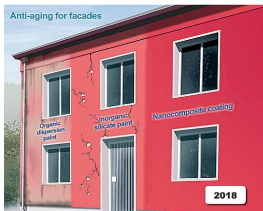
**Fig. 1** The new nanobinder Col.9 combines in one product the different advantages of conventional coating types in terms of low dirt pick-up, chalking and rack resistance, and color retention. (Reproduced from www.col9.com, with permission.)
