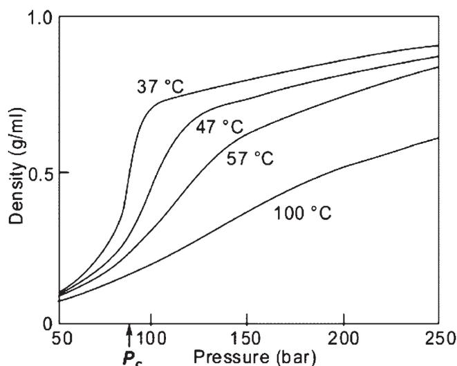
**Figure 1.** Variation of CO<sub>2</sub> density with temperature and pressure (reproduced from ref.<sup>[5]</sup> with permission).
