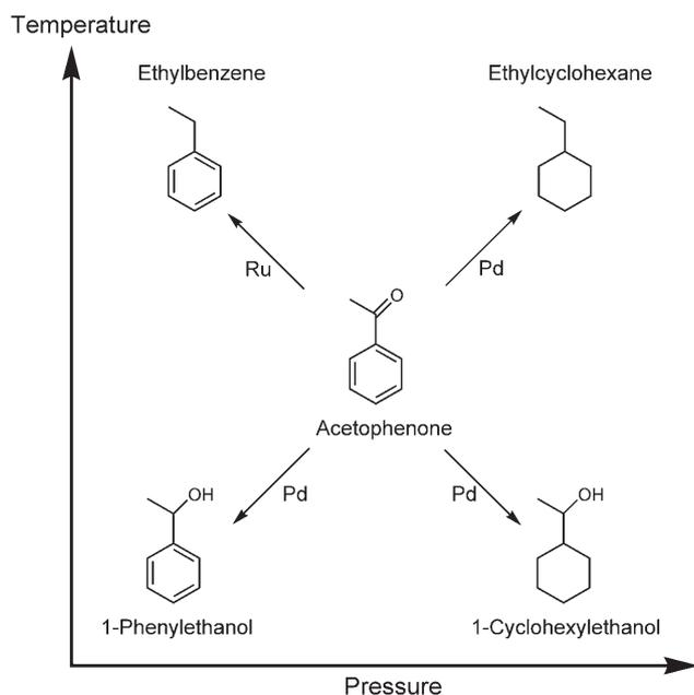
**Figure 2.** By varying temperature and pressure the selectivity of reactions in  $scCO_2$  can be largely controlled (reproduced with permission from Dr. R. Clarke, Thomas Swan Ltd.).
