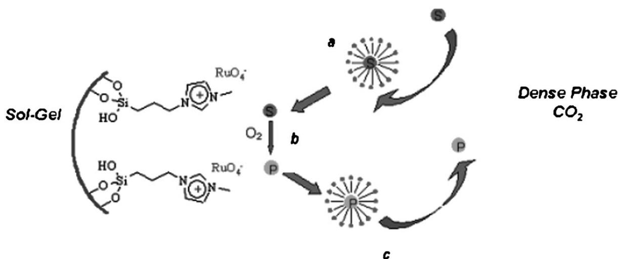
**Figure 6.** Supported ionic liquid Ru-based catalysis in  $scCO_2$  ensures smooth oxidative dehydrogenation of a variety of alcohols (reproduced from ref.<sup>[24]</sup> with permission).
