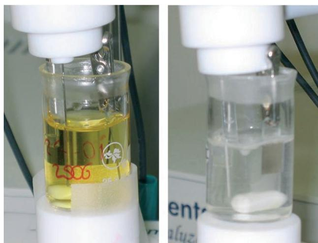
**Figure 1.** TEMPO@DE is obtained by electrodeposition of a thin layer of organosilica doped with TEMPO upon application of  $-1.1$  V (vs. Ag/AgCl) for 15 min to a solution of suitable organosilanes (left). The electrocatalytic film thereby obtained selectively converts benzyl alcohol dissolved in 0.2M NaHCO<sub>3</sub> to pure benzaldehyde by simply applying a 1.4 V voltage (right).
