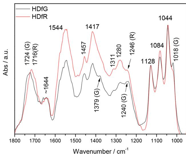
**Figure 6.** ATR spectra of the extracts obtained by hydrodiffusion after separation of pectin, normalized to the band at 1044  $\text{cm}^{-1}$ .
