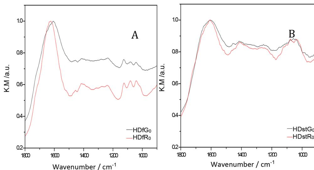
Figure 4. DRIFT spectra of the initial aqueous extracts by (A) hydrodiffusion and (B) hydrodistillation, normalized to the most intense band.
