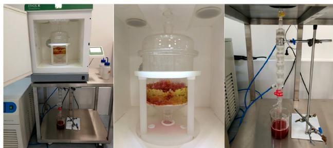
Figure 2. Ethos X extractor (left) whose vessel was filled with milled OFI peel (middle) affording the aqueous extract (right).
