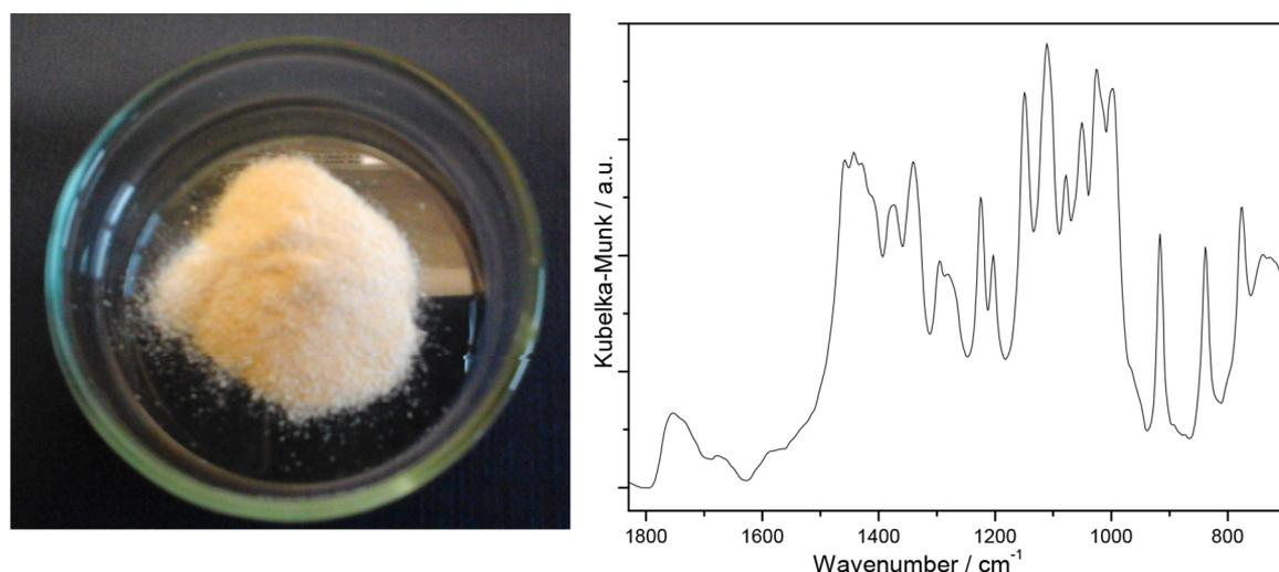
Figure 7. Pectin powder from the peel of red/green fruit and DRIFT spectrum in the fingerprint region.
