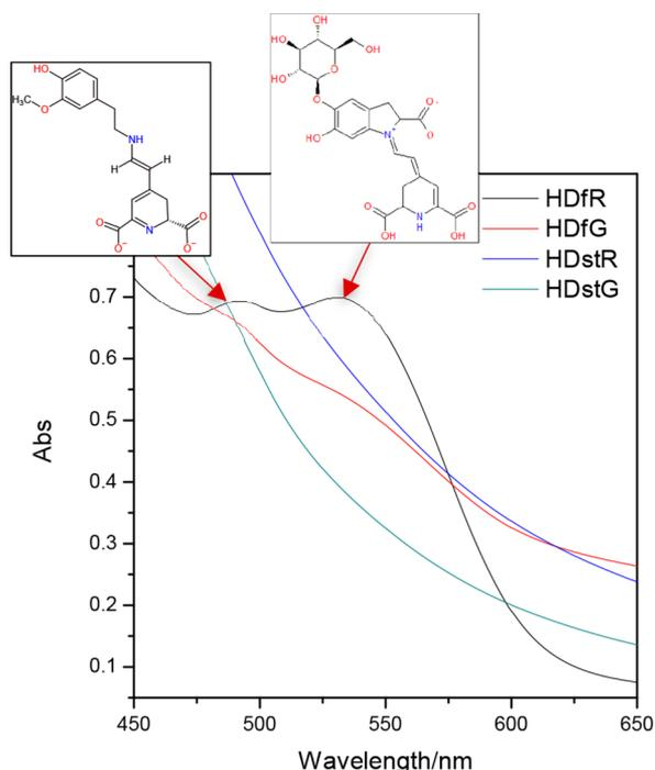
**Figure 5.** UV-vis spectra of the pectin-free solutions after a 4 month storage period for both green and red fruit peels extracted via microwave-assisted hydrodistillation and hydrodiffusion.
