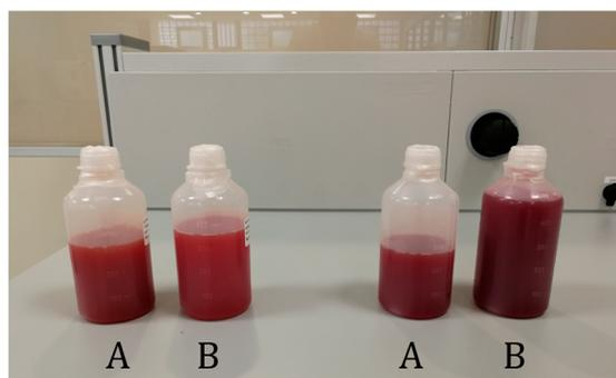
Figure 3. Aqueous extracts from green *Opuntia ficus-indica* peel (left) and from red *Opuntia ficus-indica* peel (right). (A) Samples obtained via microwave-assisted hydrodistillation. (B) Samples obtained via microwave-assisted hydrodiffusion.
