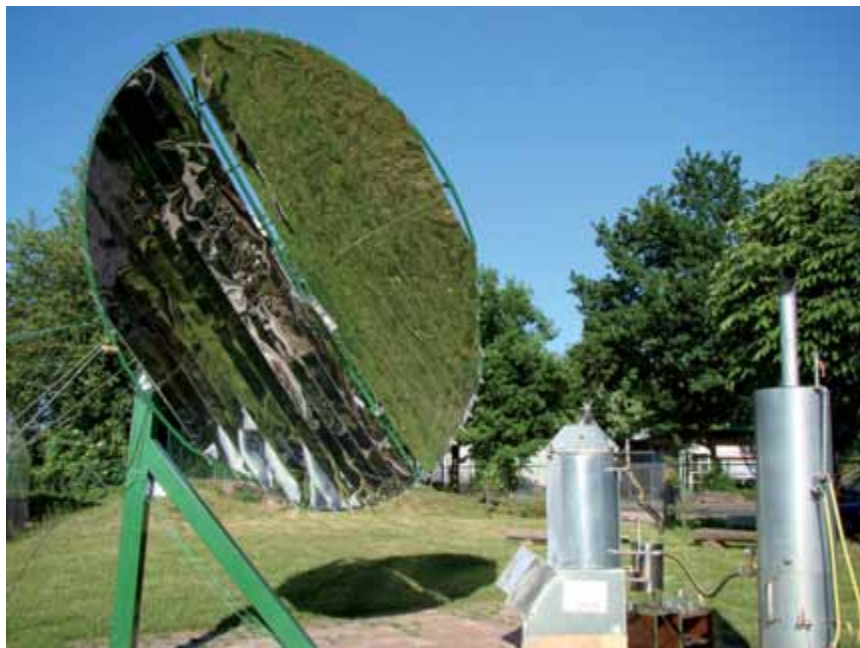
Figure 2. Solar distillation unit jointly developed at University of Agriculture Faisalabad, Pakistan, and University of Kassel, Germany. The system can provide 300-400 °C temperature (Image courtesy of Dr W. Amjad, Reproduced from Ref.7, with kind permission).
