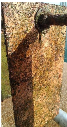
Figure 2 Right side of the shipbuilding steel substrate protected (top) by commercial topcoat and (bottom) by the AquaSun at 5 wt% bismuth tungstate load (THA8-5) after 69 consecutive days in Palermo's harbor waters.
