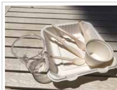
Figure 1. Single-use glass (in PLA), cup and cutlery (from starch) and plate (cellulose and another biopolymer) in biodegradable or compostable plastics used at a Sicily's lido, July 2019. A ban on non-biodegradable plastics enforced since Summer 2019 locally forbids use of conventional plastics.
