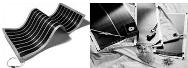
Figure 7. Plastic solar cells, such as that on the left which is entirely organic (photo courtesy of Konarka) or that on the right which uses amorphous Si (photo courtesy of Flexcell), are lightweight (25–50 g m -2 ) and ideally suited for customised integrated solutions.
