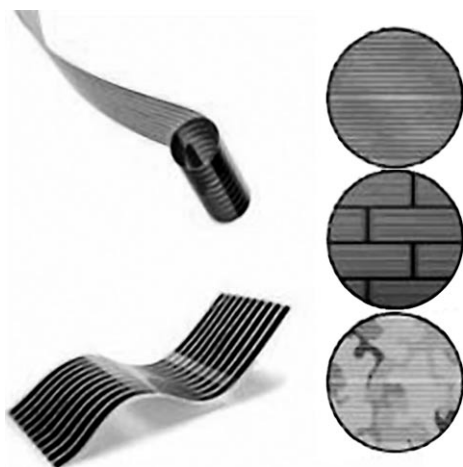
Figure 14. These rolls are commercial-grade solar photovoltaics printed by inkjet printer (image courtesy of Konarka Technologies, Inc.).
