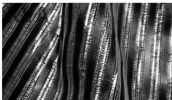
Figure 26. Top: A 3D rendering of “Soft House”, which uses household curtains to collect solar energy and provide lighting. Bottom: The flexible array of semitransparent organic photovoltaic curtains used in the Soft House; the PV cells are woven into a malleable fabric (photos courtesy of KVA MAT X).
